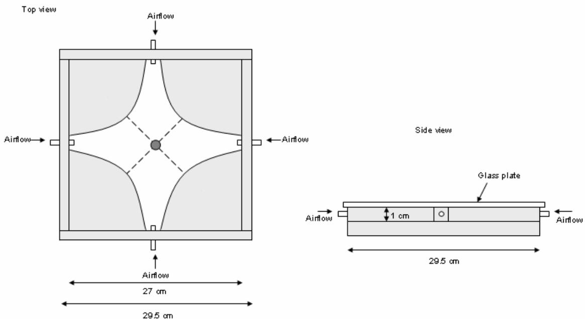
Figure 3. Schematic representation of a 4-branch olfactometer.
