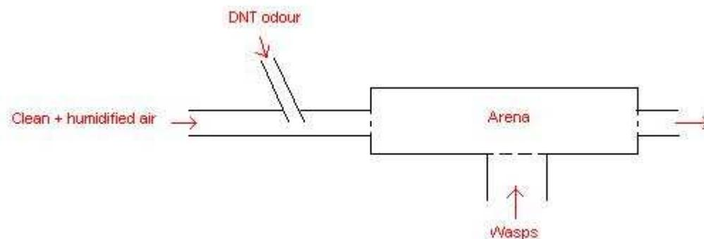
Figure 1. Schematic representation of the conditioning arena.
