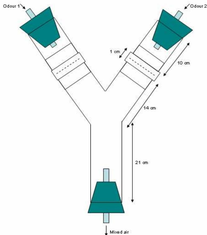
Figure 4. Schematic representation of a Y-tube.
