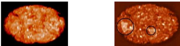
Figure 2. a) Image plane where plastic fragments are not visible b) plastic fragments (surrounded by circles) can be seen but can not be separated from fat (visible as white spots).
