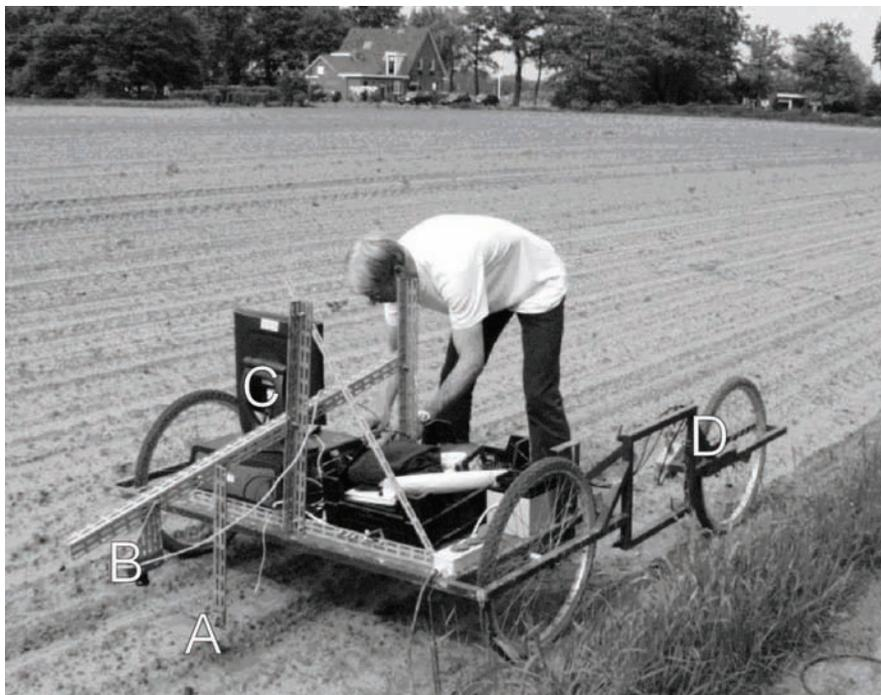
Figure 3.1 Measurement setup during the field experiment. A: Grey reference plate; B: camera; C: desktop PC; D: wheel trigger.
