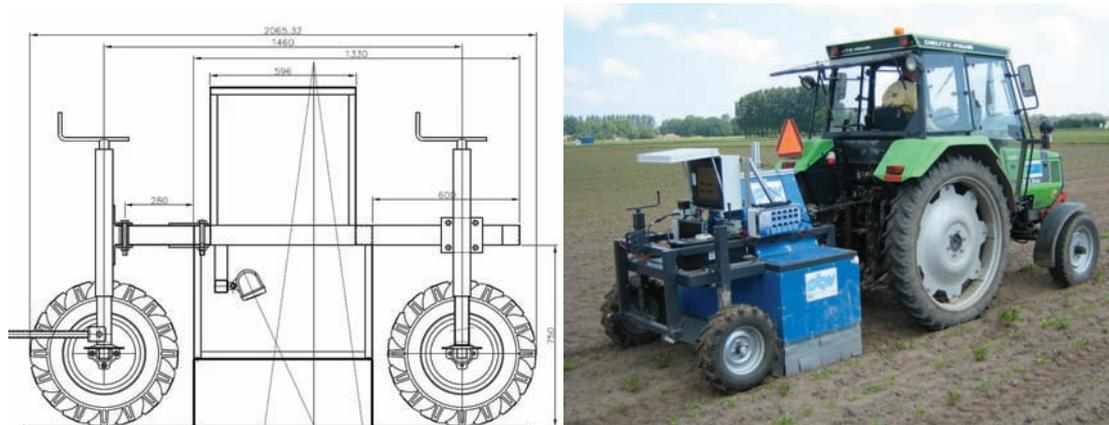
Figure 5.1 Imaging setup, (left) a schematic diagram with camera C and lamps L, (right) as used in the field attached to a tractor.
