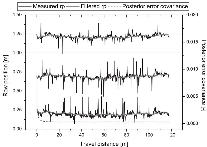
Figure 5.9 Measured row position (rp) and filtered row positions and the posterior error covariance at 28-05-2008 on clay soil as function of the travelled distance.
