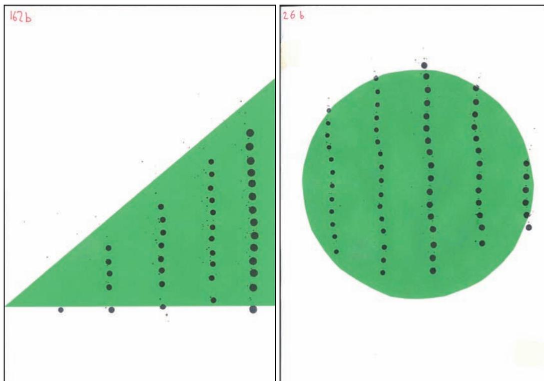
Figure 8.7 Example scanned image of sprayed triangle (a) and circle (b). Five rows of droplets were sprayed. The targets were placed on A4 paper (21x29.7 cm)
