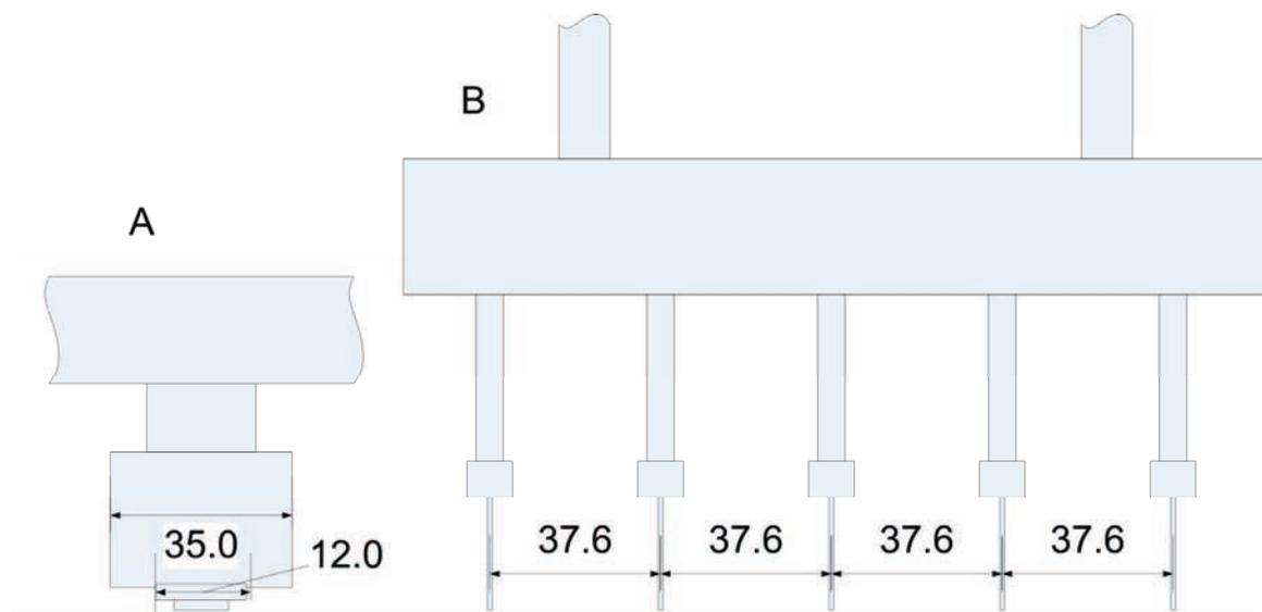
Figure 7.2 Schematic scale presentation shows the dimensions of the micro-sprayer (B) compared to the standard TeeJet XR11004 flat fan nozzle(A). Dimensions have unit [mm].
