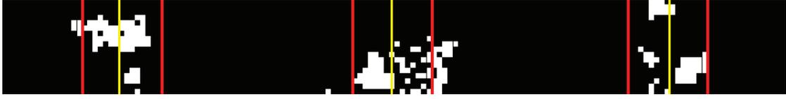
Figure 5.8 Row detection results overlaid on the vegetation grid cells image. The yellow lines represent the crop row position, the red lines represent the crop row width.
