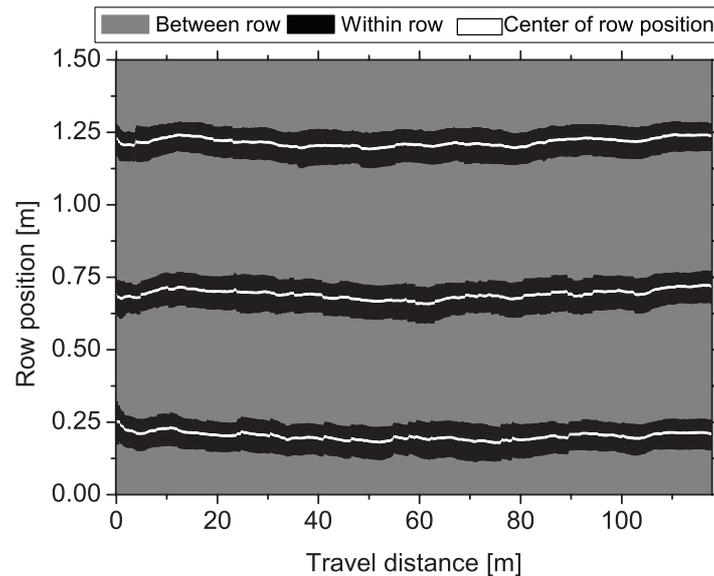
Figure 5.11 Row position and row width are given as a function of the travel distance. The black areas within the crop row were used as training data for sugar beet plants, the grey areas were used as training data for volunteer potato plants.
