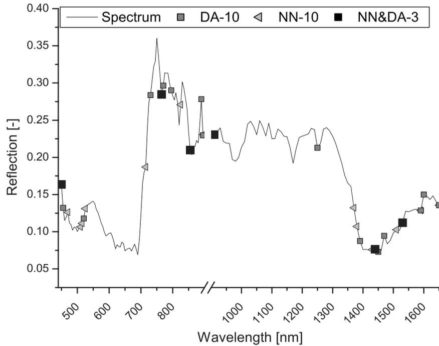
Figure 2.3 Selected discriminative wavelength bands shown on an arbitrary measured spectrum. On the left of the x-axis break the selected bands for sensor 1, on the right the bands for sensor 2. DA-10: 10 fixed wavebands for discriminant analysis selection method, NN-10: 10 fixed wavebands for neural network selection method, NN&DA-3: 3 fixed wavebands that were selected by both the neural network and the discriminant analysis.
