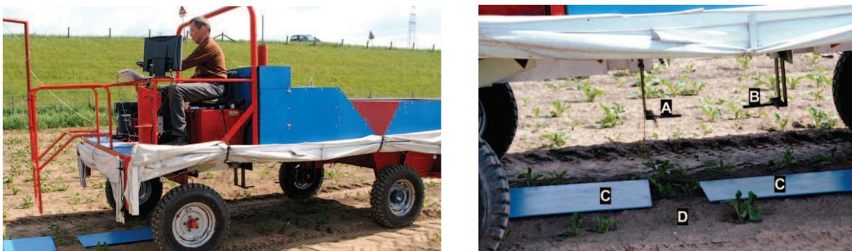
Figure 2.1 InspectorMobile measurements in a sugar beet field. A and B are reflectance references in the field of view of sensor 1 and sensor 2 respectively. C are plastic sheets covering vegetation that was not recorded. D is one of the plants recorded by sensor 1.
