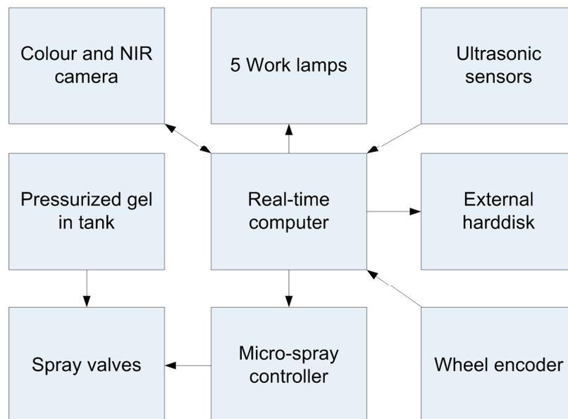
Figure 8.1 Schematic overview of the system components. The arrows indicate the uni- or bidirectional connections between the system components.
