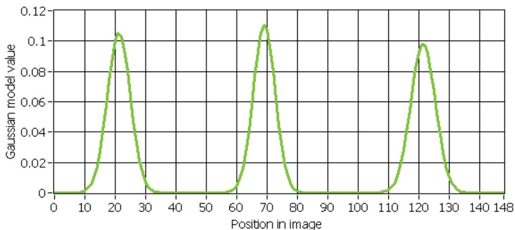
Figure 5.7 Fitted Gaussian bell shapes on the histogram of vegetation grid cells. Mean and standard deviation of normal distribution represents row position and row width.
