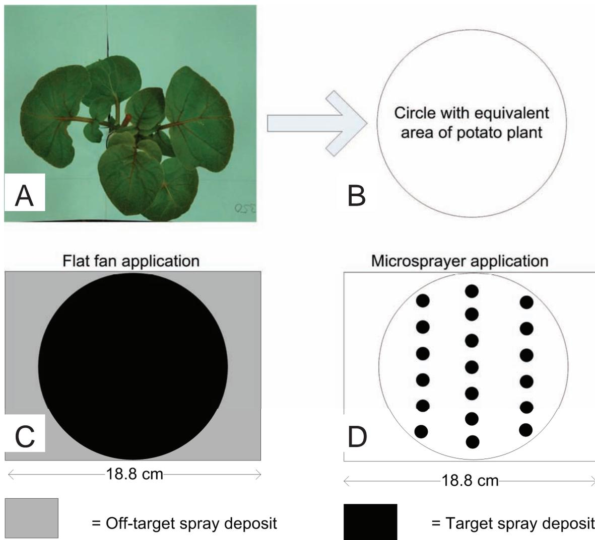
Figure 7.4 Scheme showing calculation of off-target spraying. a) Ground covered surface area determination of potato plant. b) Area is transformed to a circle. c) Flat fan application showing off-target spray deposition. d) Microsprayer application spraying drops on demand within the contours of the plant.
