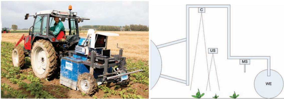
Figure 8.2 Measurement setup in arable field conditions. Two cameras and five xenon work lamps are located under the blue cover with grey plastic flaps. On the system two cameras (C), ultrasonic sensors (US) the microsprayer (MS) and wheel encoder (WE) are connected. The microsprayer consists of five needles and has a working width of 20 cm.
