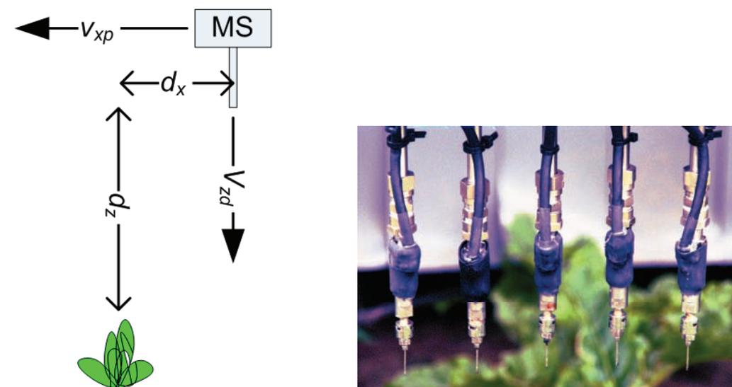
Figure 8.4 Schematic of the micro-sprayer (MS) above the weed potato plants to be sprayed. The micro-sprayer is connected to the platform as shown in (B) and moves forward with platform velocity in x-direction  $v_{xp}$ . The droplets released from the micro-sprayer have a velocity in the z-direction  $v_{zd}$ . The vertical distance between needle and weed potato plant is  $d_z$ . The droplet release distance in travel direction is  $d_x$ .
