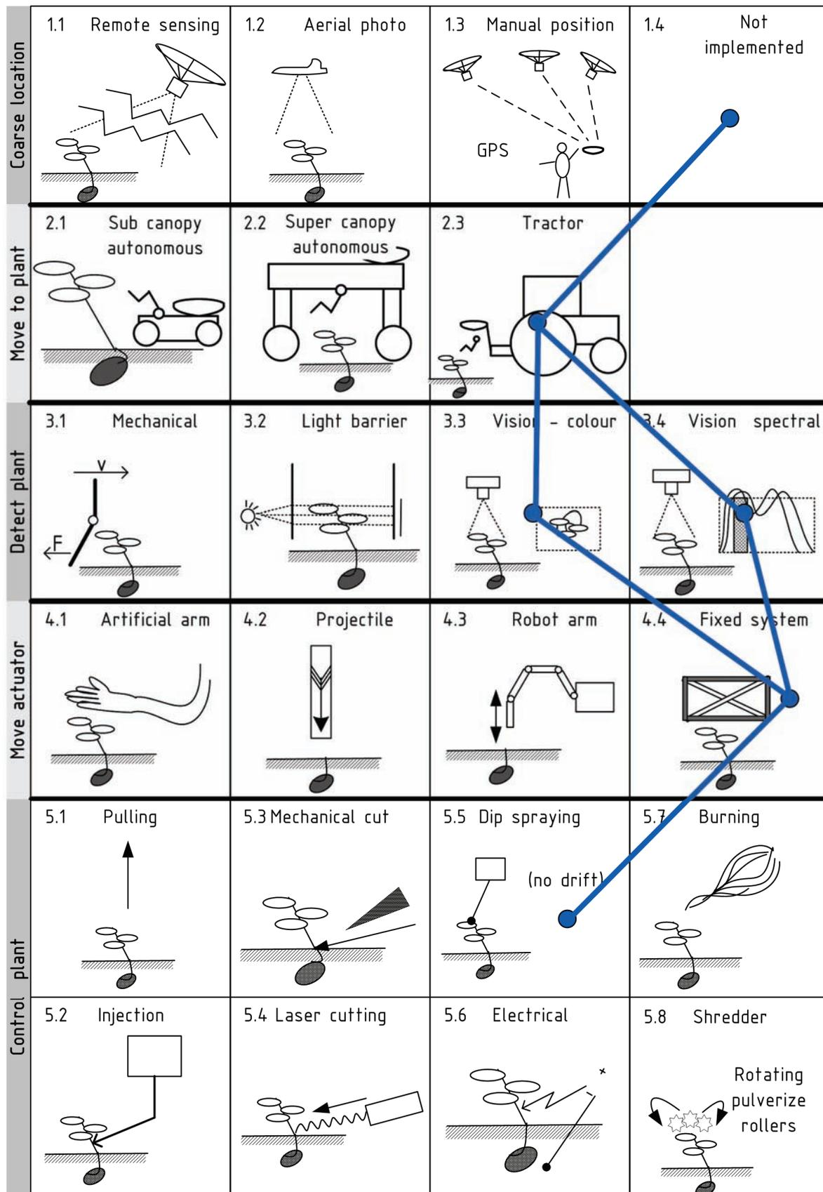
Figure 1.1 Part of the morphologic chart. The five functions are shown in the leftmost column. Possible methods to fulfill a function are shown with a pictogram. From the methods a combination was chosen as a structure indicated with the line.
