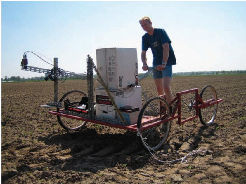
Figure 4.1. Manually operated mobile measurement setup with row recognition camera (R) and crop recognition camera (C). The field of view of the row recognition camera has an overlap of 0.1 m with that of the crop recognition camera.
