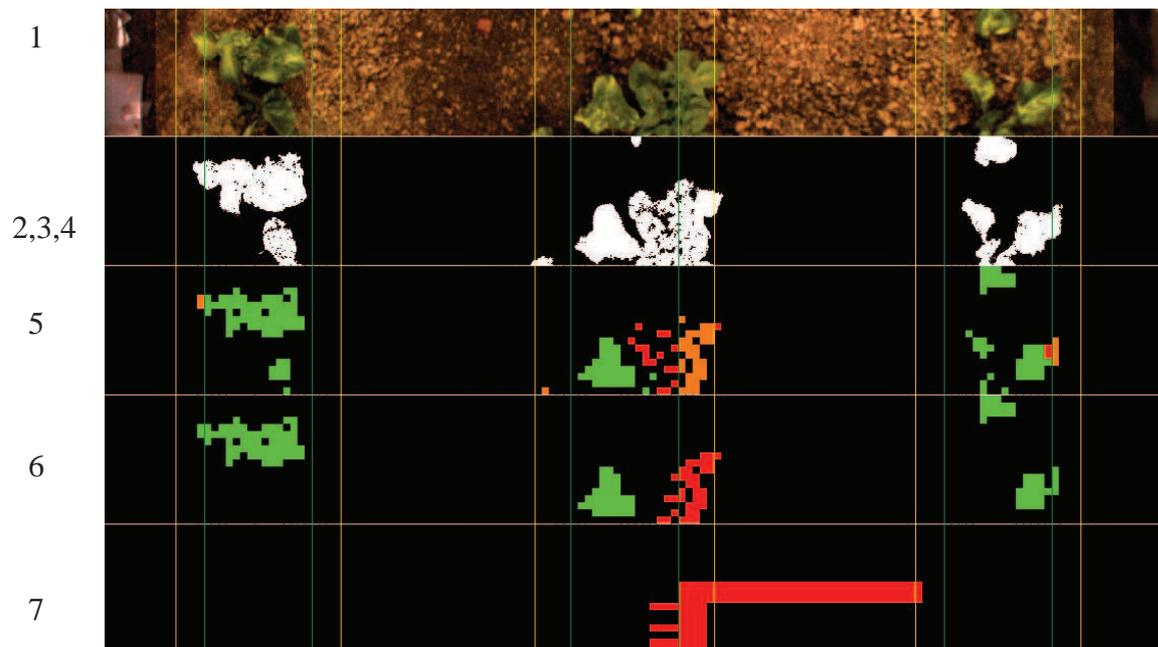
Figure 8.3 Image processing steps. Top image dimensions are 150 cm width and 20 cm length, three sugar beet rows with a row spacing of 50cm are in the field of view. 1) colour image is recorded 2, 3, 4) vegetation and crop rows are detected, colour features extracted, and classifier is trained 5) vegetation is classified 6) small plants are filtered 7) spraying decision are made.
