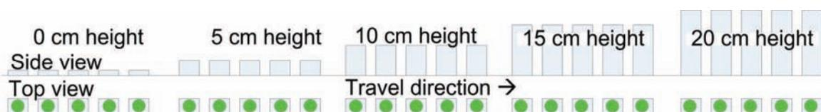
Figure 8.6 Experimental setup during accuracy testing of the precision spraying equipment. The top-view shows the position of the  $254 \text{ cm}^2$  circles on A4-paper ( $21 \times 29.7 \text{ cm}$ ) that were used as targets.
