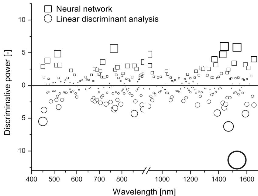
Figure 2.2 The normalized discriminative power between sugar beet and potato reflectance spectra of a specific band is shown as a function of all measured wavelength bands. Larger bubbles and squares indicate larger discriminative power for the linear discriminant analysis and neural network respectively. Results for the “10 optimal” wavebands for the 15 datasets.
