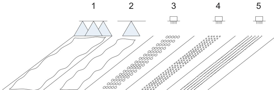
Figure 7.1 Schematic overview of the five treatments were done on the spray track. Treatment 1: a conventional spray fluid sprayed by three flat fan nozzles. Treatment 2: a gel fluid sprayed by one flat fan nozzle. Treatment 3: a low droplet density pattern of gel sprayed by a micro-sprayer. Treatment 4: a medium droplet density pattern of gel sprayed by a micro-sprayer. Treatment 5: a high droplet density pattern of gel sprayed by a micro-sprayer.
