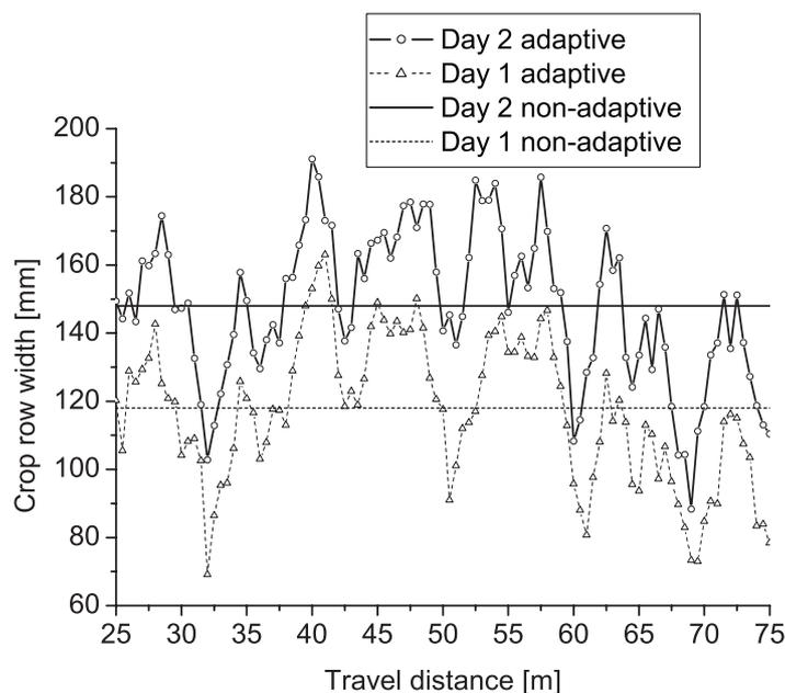
Figure 4.4 Crop row width [mm] as a function of travel distance [m] during the two experiments.
