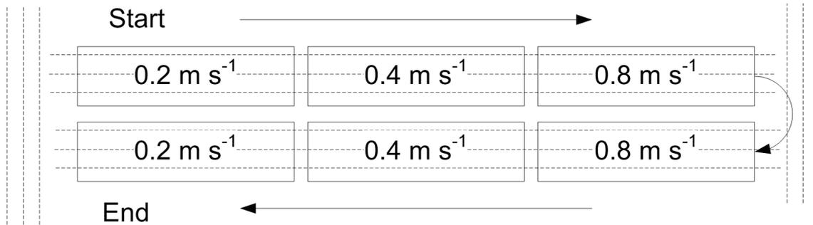
Figure 8.5 Schematic of the experimental field. Sugar beet rows are indicated with - - - . Travel velocity was increased while driving in one direction and was decreased while travelling back. Three sugar beet rows were covered by the system. The headlands were not used during the experiment.
