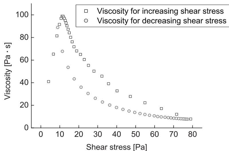
Figure 7.3 Relation between shear stress and viscosity of the gel fluid as used in the micro-sprayer. The relation was measured with a rheometer, the temperature of the gel was 20 °C during the measurement.
