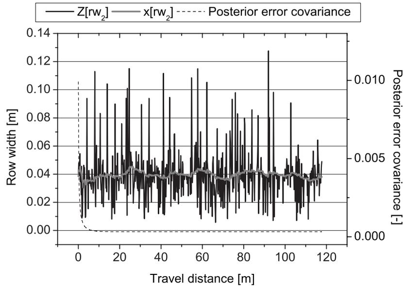
Figure 5.10 Measured row width of the middle row ( $Z[rw_2]$ ) and filtered row width of the middle row ( $x[rw_2]$ ) and the posterior error covariance at 28-05-2008 on clay soil as function of the travelled distance.
