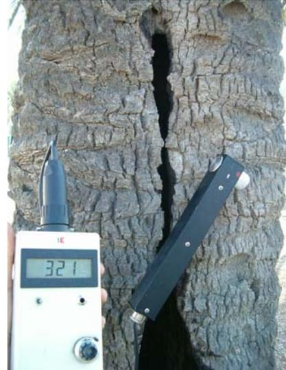
**Figure 3.** Extraordinary shearing deformations (in 1/1000 mm), in comparison with pure longitudinal fibre elongations, suggest sliding over each other of the two halves of the stem
