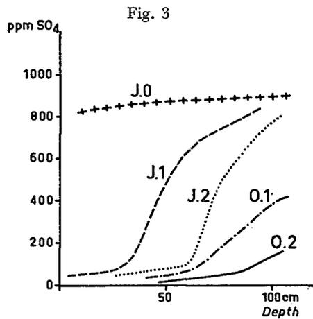
Fig. 3. Approximate  $\text{SO}_4$  content (in Morgan-Venema extract) in profiles of the landscapes as recognized.
