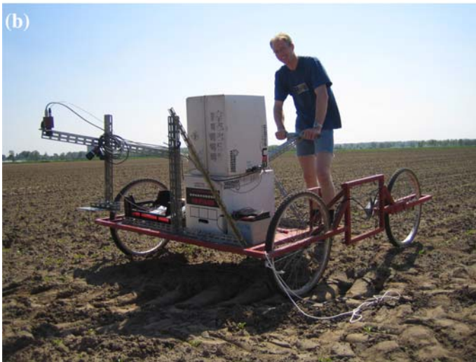
Fig. 1 Manually operated mobile measurement setup with row recognition camera (R) and crop recognition camera (C). The field of view of the row recognition camera has an overlap of 0.1 m with that of the crop recognition camera
