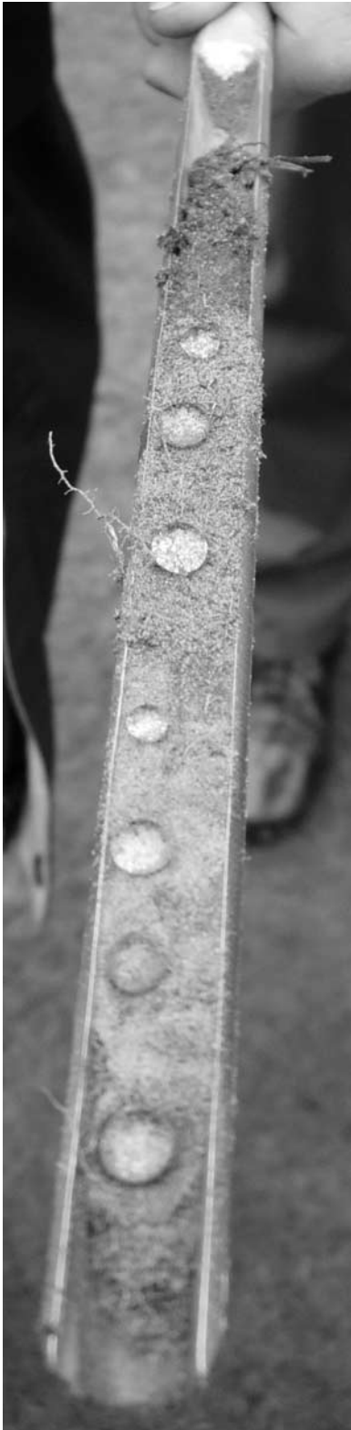
Figure 1. Soil core sampler containing a 25-cm-long water repellent sandy column, as shown by the water drops remaining on the soil surface.
