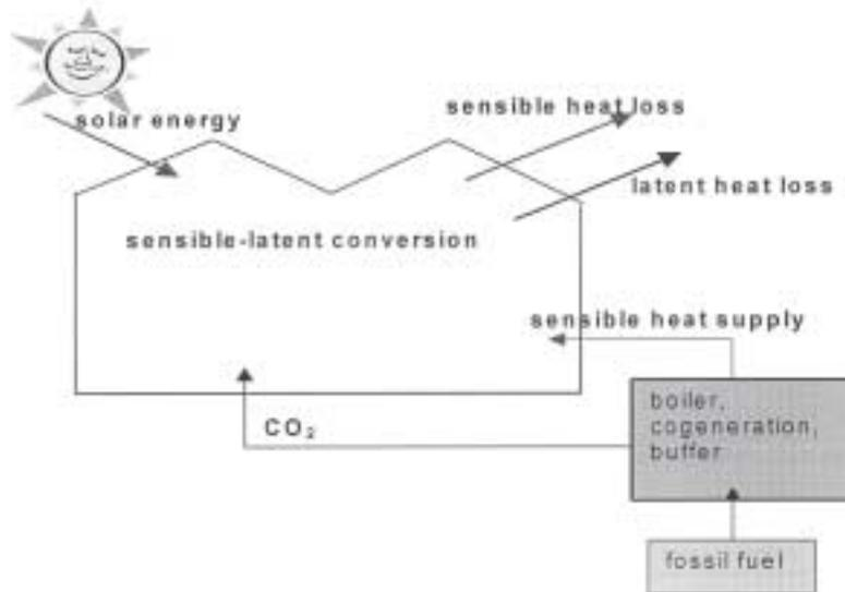
Fig. 1. Energy scheme of a conventional greenhouse
