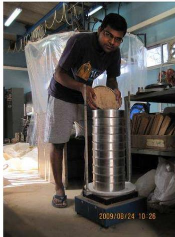
**Figure 6: Pouring the sample on the top nest for sieving**
