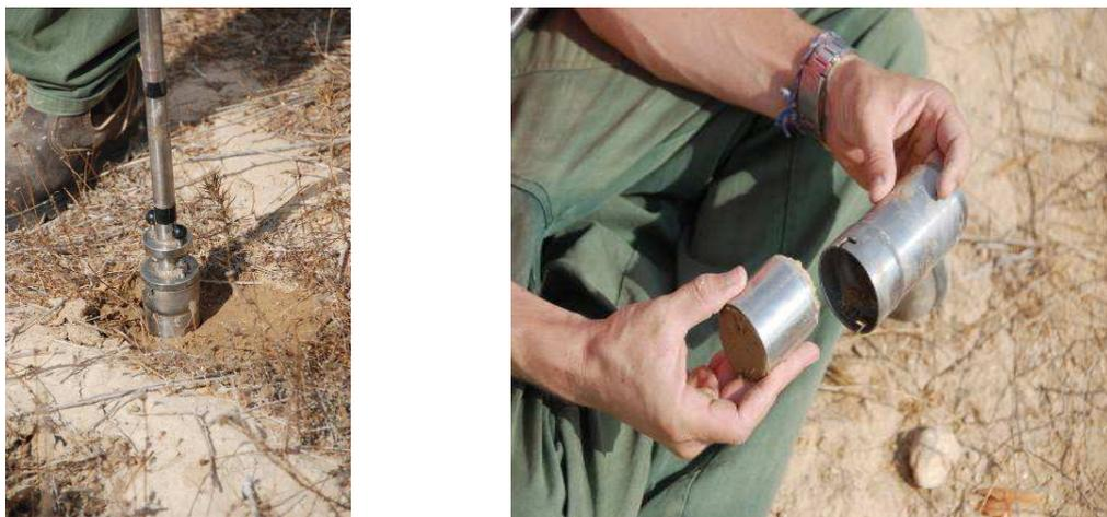
**Figure 5: Left - sampling with soil core sampler, Right - sample removed from the cylinder**
