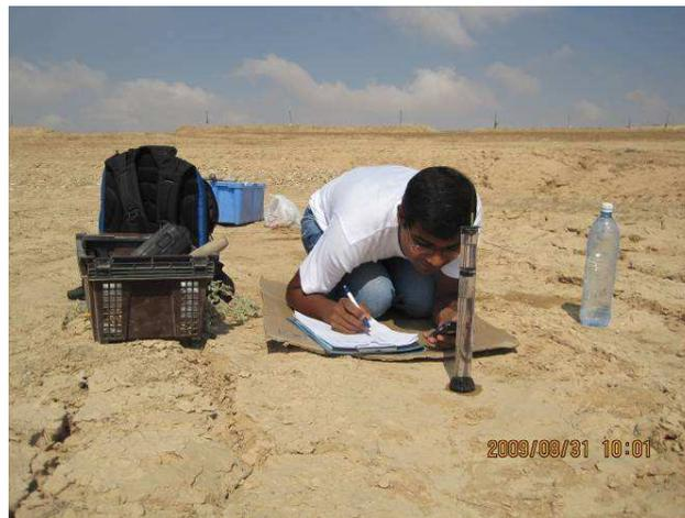
**Figure 7: Taking reading for the infiltration rate**
