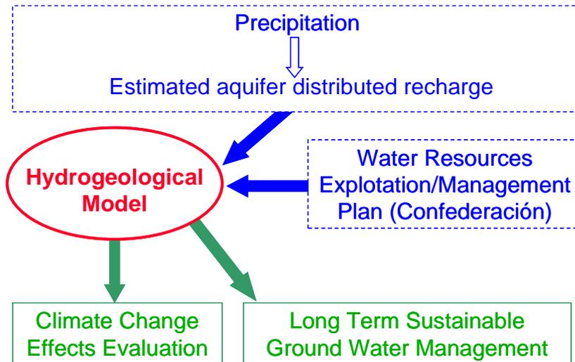
Figure 3.2: Flow diagram for assessing the changes driven by the climate change in the groundwater resources. Blue dashed lines are input data for the Hydrogeological model, and green solid lines are output data.
