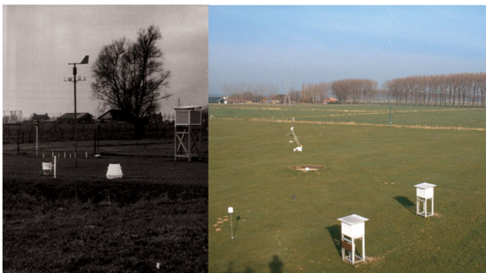
Figure 1. Left panel: overview of one of the first designs of the Wageningen University meteorological observatory. In the centre is the tilting-siphon rain recorder set-up. Right panel: overview of the current set-up of the observatory. In the centre is the turf wall grass rain gauge set-up. This figure is available in colour online at www.interscience.wiley.com/ijoc
