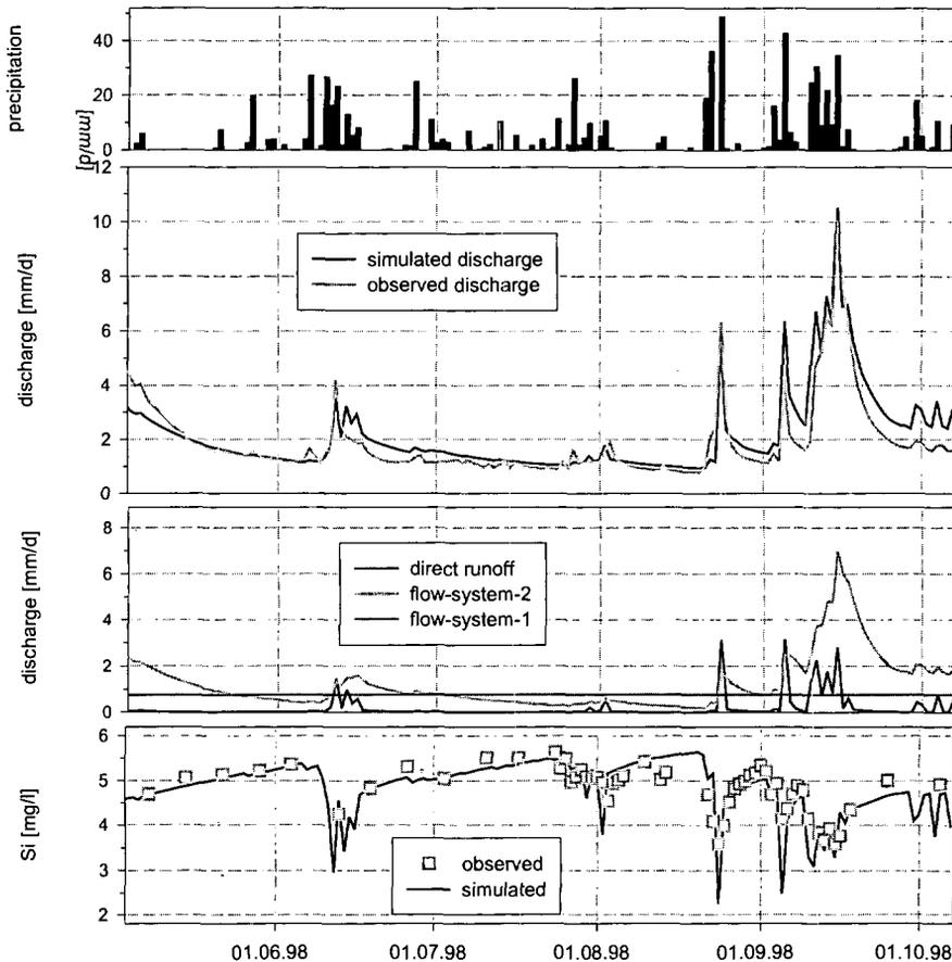
**Figure 3:** Measured basin wide precipitation (first), comparison of simulated and observed discharge at the Brugga gauging station (second), portions of the different runoff components (third) and comparison of observed and simulated dissolved silica concentrations (observed concentrations with error bars; fourth) for the period 03.05.98–07.10.98 (adapted from Uhlenbrook et al., 2000).
