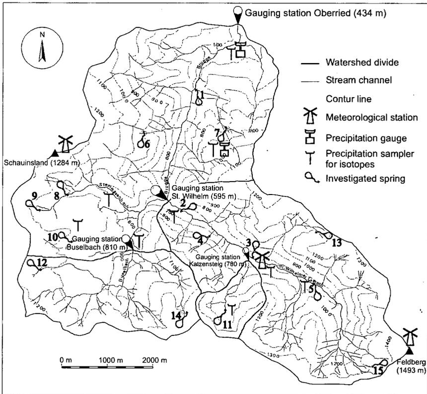
**Figure 1:** Schematic sketch of the Brugga basin with instrumentation and investigated springs (adapted from Uhlenbrook and Leibundgut, 2001).
