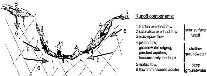
**Figure 2:** Schematic depiction of the runoff generation at the test site (adapted from Uhlenbrook and Leibundgut, 2000).
